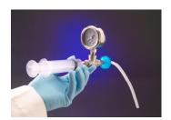
Note: The following procedure was developed for testing HP1002 0.2µ filters. Refer to a filter manufacturer's specifications when testing any other filter.
